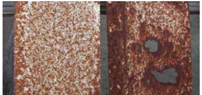
Galvanised Steel Z300 Washed Panels – Exposed for 21 years
